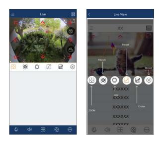
Please control the PTZ by sliding the image in direction of the arrow marked on the image. The PTZ will automatically focus on the little red circle by clicking the image. Then the 3D function can be enabled (the added device must support 3D function, or this function is ineffective).
