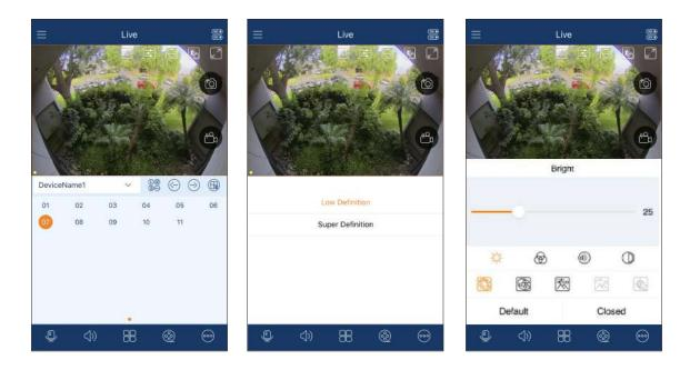
Fisheye mode. This icon appears only when this channel is a fisheye camera. Click this icon to go to fisheye display mode as shown below. Different view modes can be selected in this interface.
