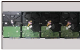
2. Screw the screws into the HDDs and fix the HDDs onto the mounting bar.
