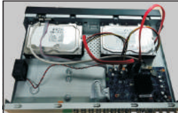
4. Connect the power and data cables.
