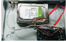
4. Connect the power and data cables.
