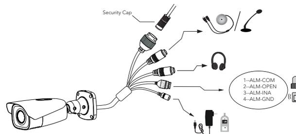
\*1 It is recommended to install the security cap for outdoor installation.
