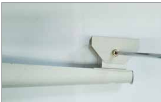
1. Remove 2 bolts and detach bracket-shoulder from wall mount arm.
