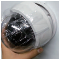
5. Close the cover to complete installation
