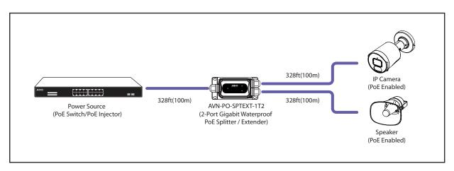
AVN-PO-SPTEXT-1T2 divides up to 90W of power between two PoE devices allowing seamless integration by transmitting both power and data. Ideal when adding another PoE device such as IP speaker or camera using one cable with same power source.
